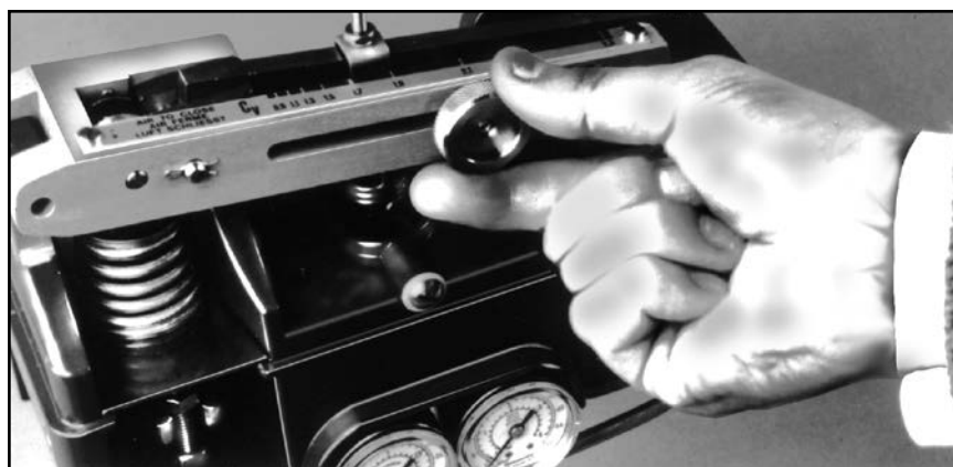
Figure 3: Flow Coefficient Adjustment
