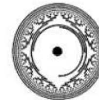
Rotary disc of an absolute encoder.
