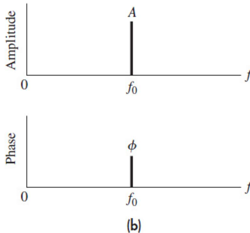
Representations of  $A \cos(\omega_0 t + \phi)$ : (a) phasor diagram; (b) line spectrum. <sup>3</sup>
