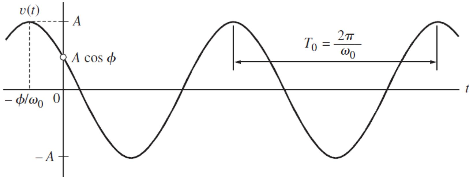
A sinusoidal waveform  $v(t) = A \cos(\omega_0 t + \phi)$ .
