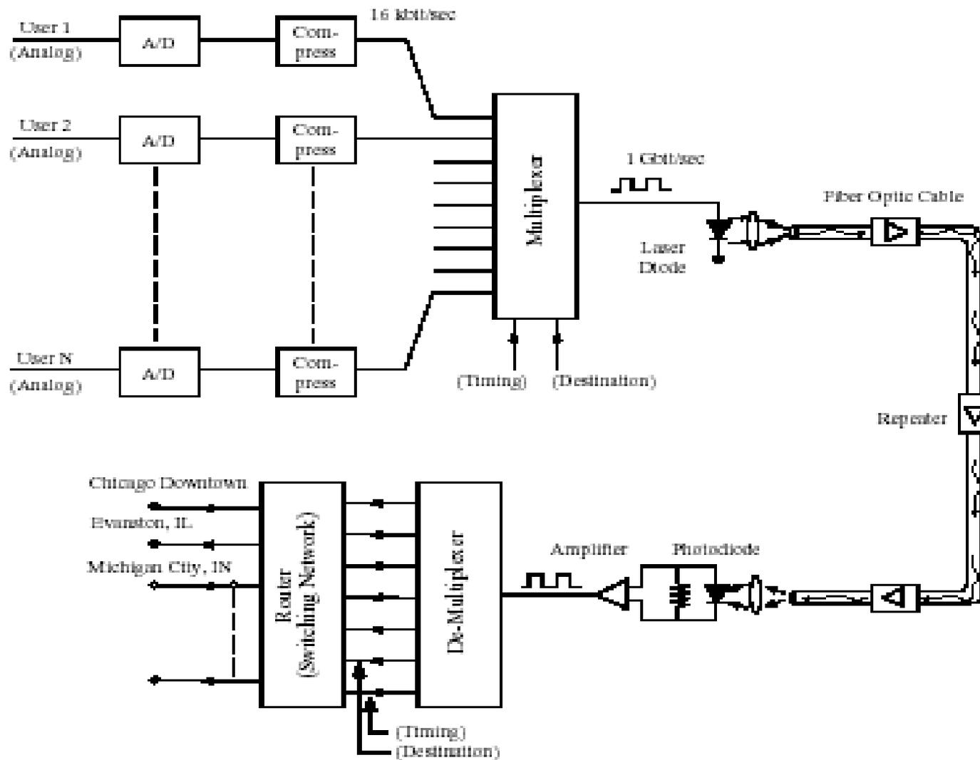
Figure 6: The optical digital telephone system.
