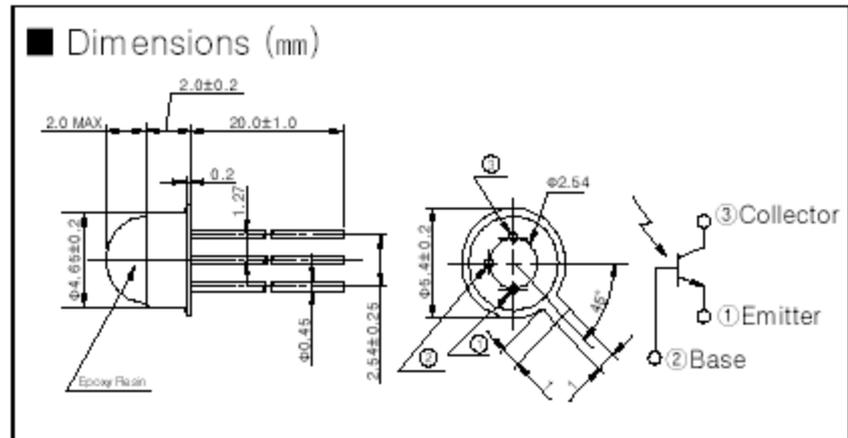
**Plastic Fiber Optic Phototransistor Detector
