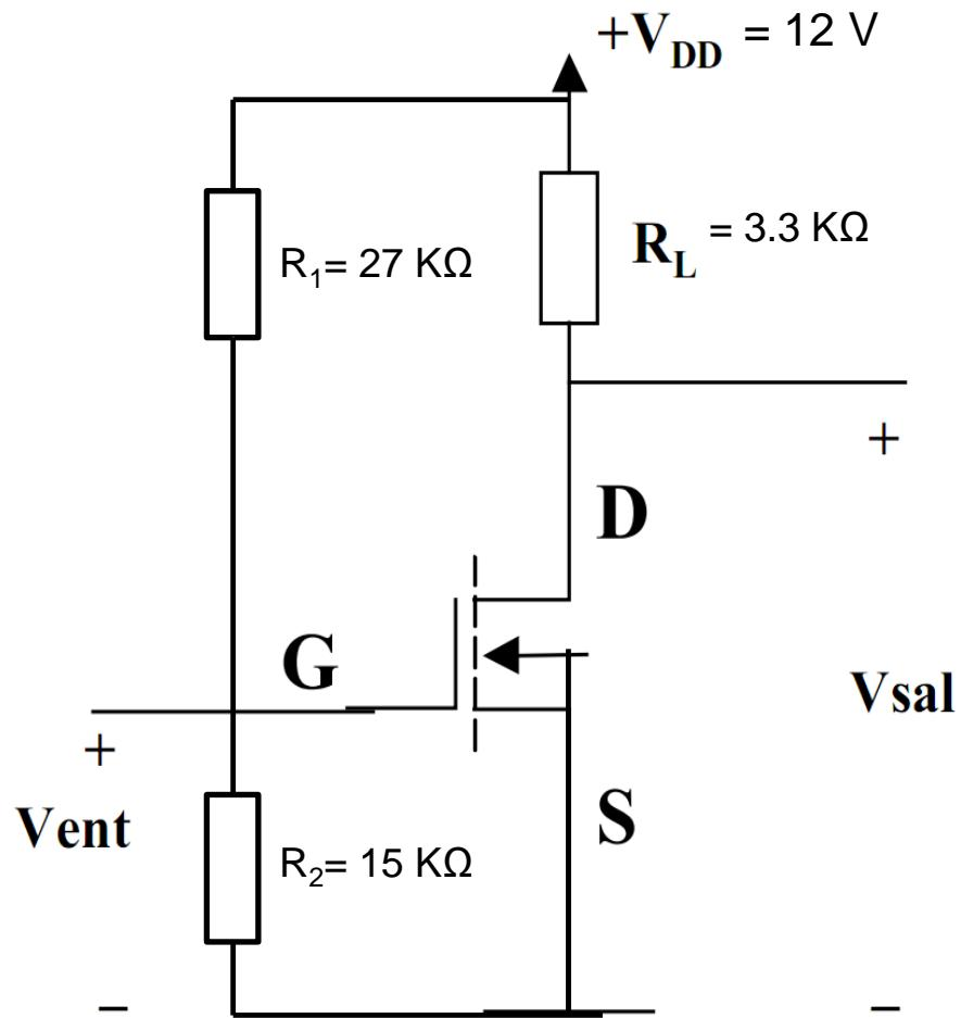
$$V_{GS} = \frac{V_{DD} \times R_2}{R_1 + R_2} \quad V_{GS} = 4,28 \text{ V}$$
