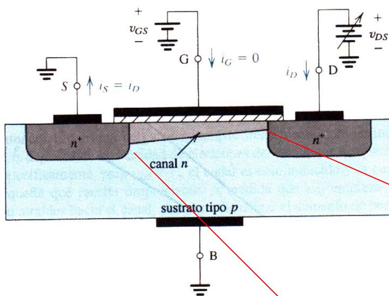
$$I_{DS} = \beta (V_{GS} - V_{TH}) V_{DS} - \frac{\beta}{2} V_{DS}^2$$
