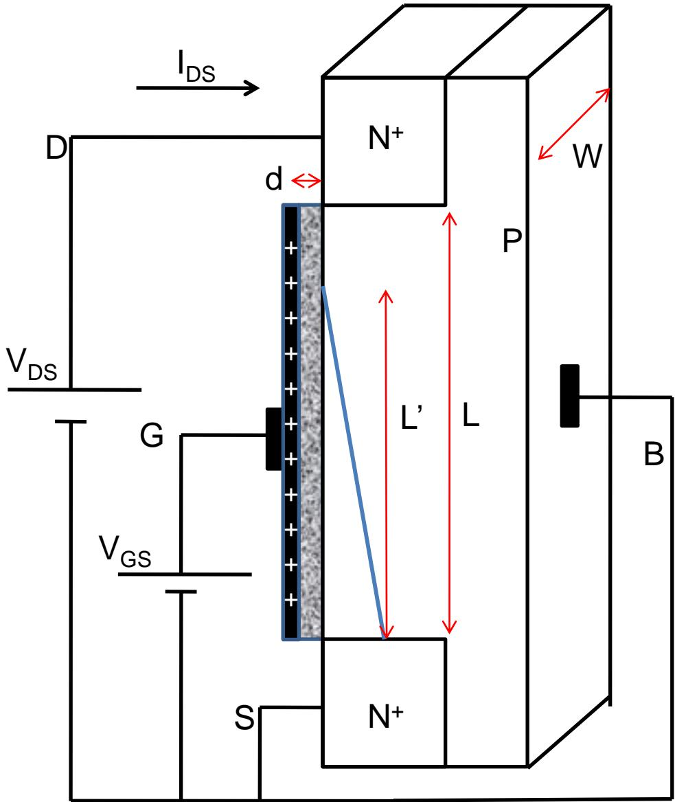
$$I_{DS} = \frac{\beta}{2} (V_{GS} - V_{TH})^2$$
