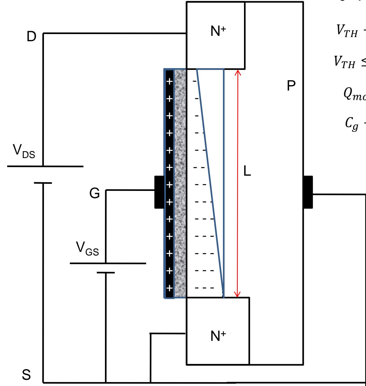
$$0 < V_{GS} < V_{TH} \rightarrow Q_{movil} = 0$$
