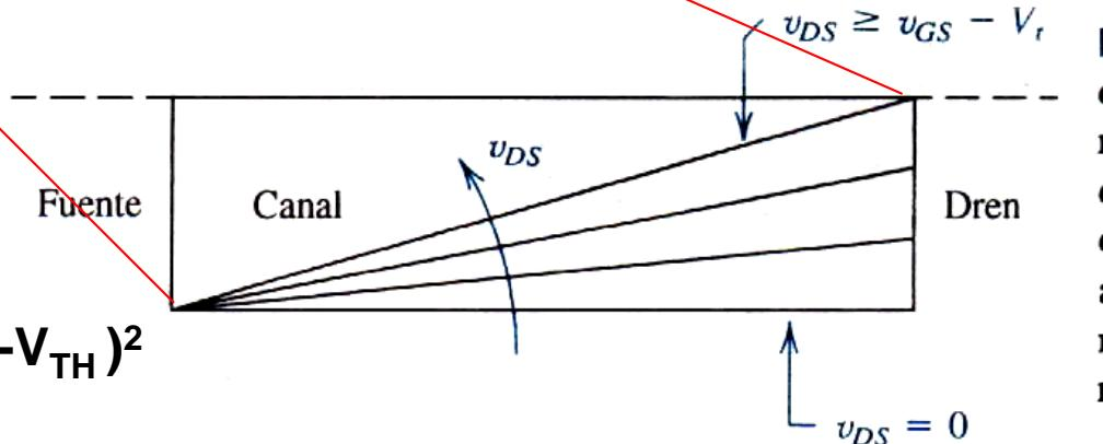
$$I_{DS} = \beta (V_{GS} - V_{TH}) (V_{GS} - V_{TH}) - \frac{\beta}{2} (V_{GS} - V_{TH})^2$$
