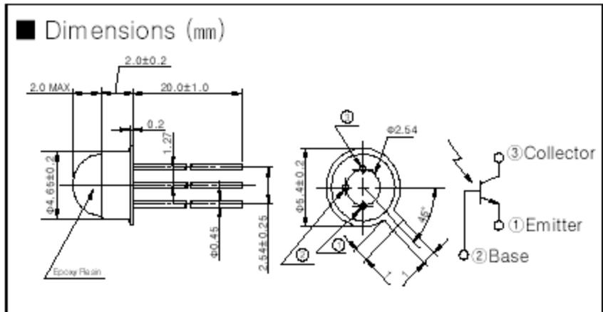
**Plastic Fiber Optic Phototransistor Detector
