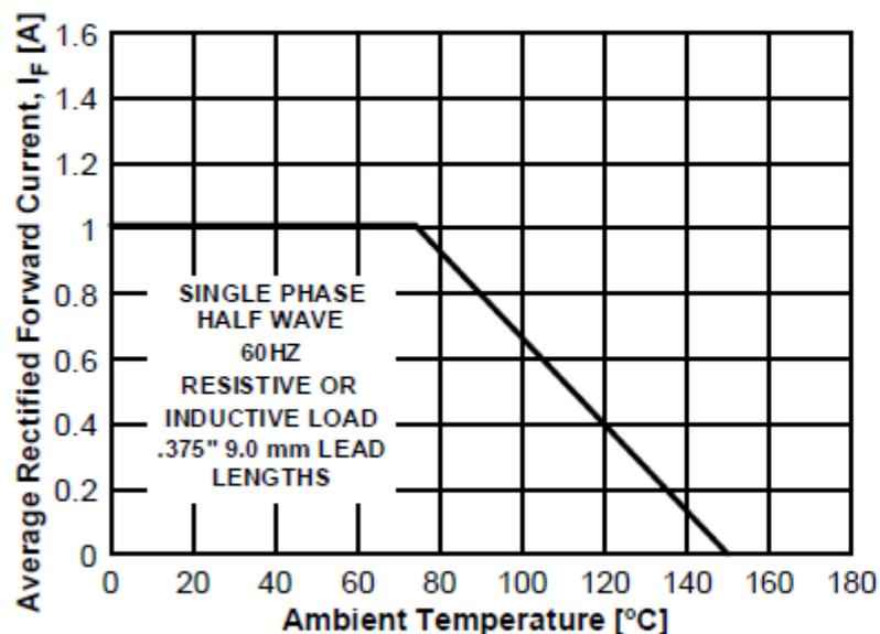
Figure 1. Forward Current Derating Curve
