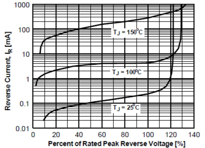
Figure 4. Reverse Current vs Reverse Voltage
