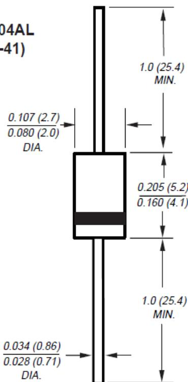
NOTE: Lead diameter is  $\frac{0.026 \text{ (0.66)}}{0.023 \text{ (0.58)}}$  for suffix "E" part numbers
