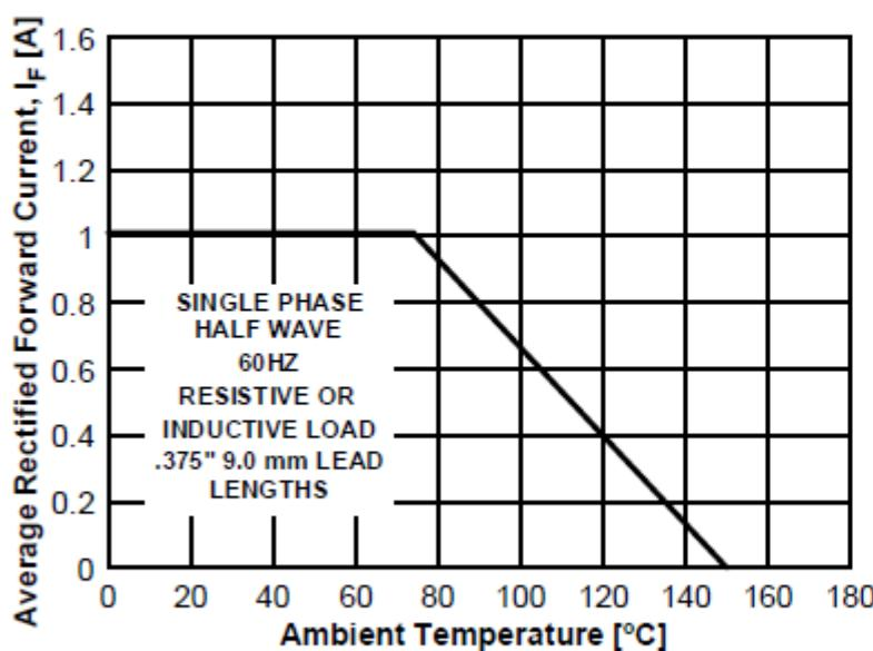
Figure 1. Forward Current Derating Curve
