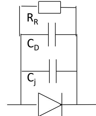
$$Q \text{ (Factor de calidad)} = \omega (C_D + C_j)(R_R \parallel r_d)$$
