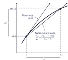
$$v(t_{i+1}) = v(t_i) + \left[ g - \frac{c_d}{m} v(t_i)^2 \right] (t_{i+1} - t_i)$$
