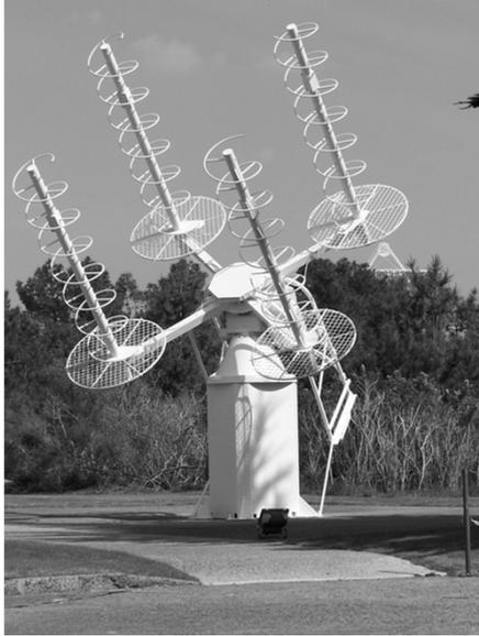
Array of four axial-mode helical antennas used as a satellite tracking-acquisition antenna, Pleumeur-Bodou, France
