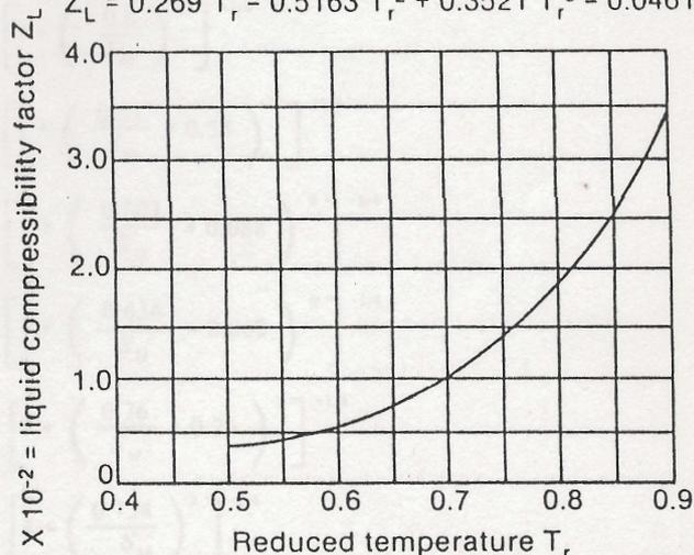
**Figure 10-12. Generalized Liquid Compressibility Factor**
