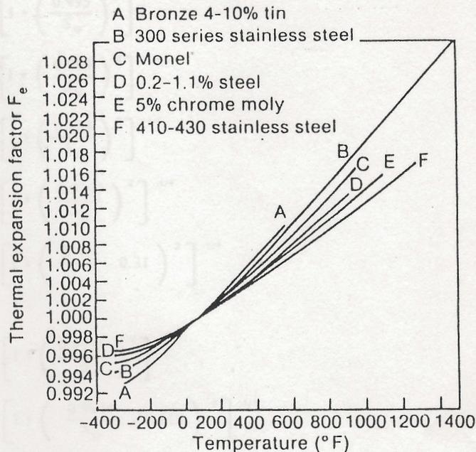
**Figure 10-11. Thermal Expansion Factor  $F_e$ .**
