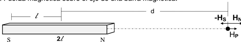
$$H_P = H_P = H_N + (-H_S) = m/(d-l)^2 - m/(d+l)^2 = [m(d^2+2dl+l^2) - m(d^2-2dl+l^2)] / (d^2-l^2)^2$$
