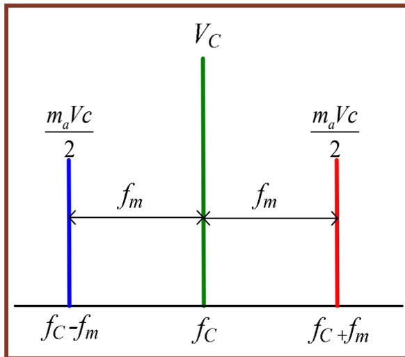
$$V_{BLS} = V_{BLI} = \frac{m_a V_c}{2}$$
