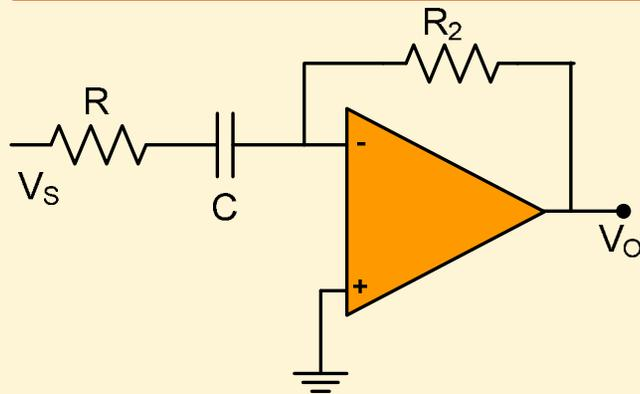
$$|A_v| = \frac{R_2}{R_1} \frac{1}{\sqrt{1 + \left(\frac{\omega_c}{\omega}\right)^2}} = \frac{A_o}{\sqrt{1 + \left(\frac{\omega_c}{\omega}\right)^2}}$$
