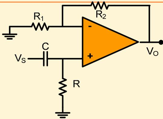
$$|A_v| = \left(1 + \frac{R_2}{R_1}\right) \frac{1}{\sqrt{1 + \frac{1}{\omega^2 C^2 R^2}}} = \frac{A_o}{\sqrt{1 + \left(\frac{\omega_c}{\omega}\right)^2}}$$
