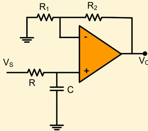
$$|A_v| = \left(1 + \frac{R_2}{R_1}\right) \frac{1}{\sqrt{1 + \omega^2 C^2 R^2}} = \frac{A_o}{\sqrt{1 + \omega^2 / \omega_c^2}}$$
