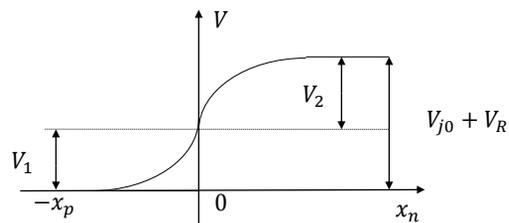
$$V_1 + V_2 = V_{j0} + V_R = -V_{j0} + V_D$$
