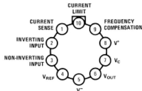
Note: Pin 5 connected to case.
