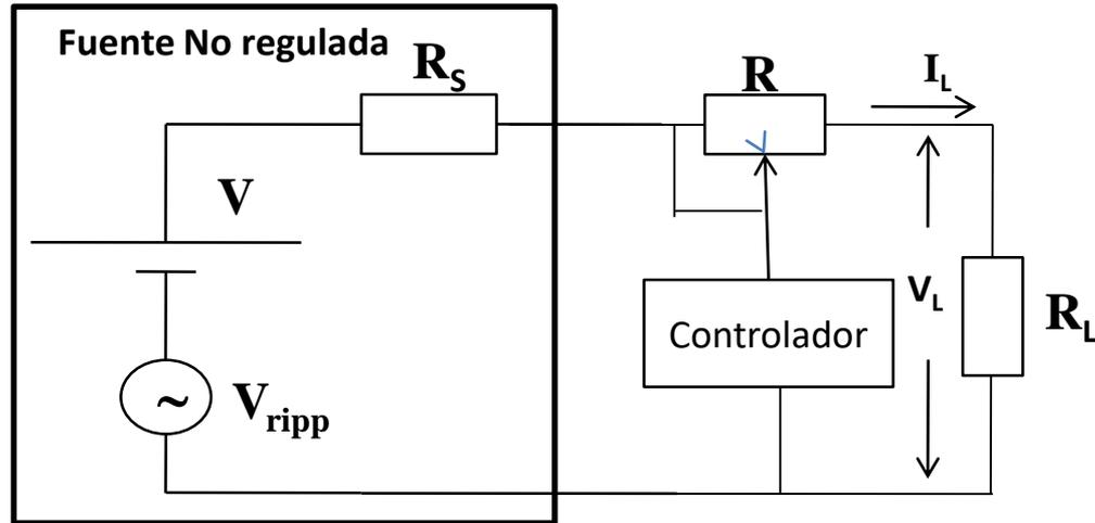
$$V_L = \frac{V * R_L}{(R + R_s + R_L)}$$
