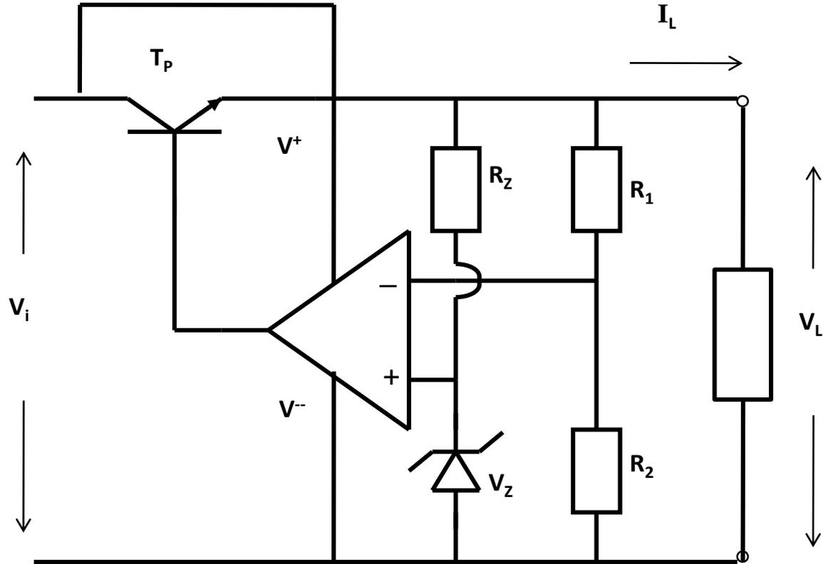
$$k = \frac{R_2}{R_1 + R_2}$$
