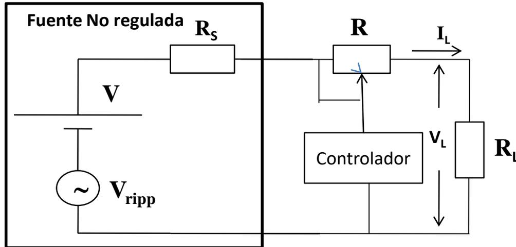
$$V_L = \frac{V * R_L}{(R + R_s + R_L)} \quad \text{si } (R + R_L) \gg R_s$$
