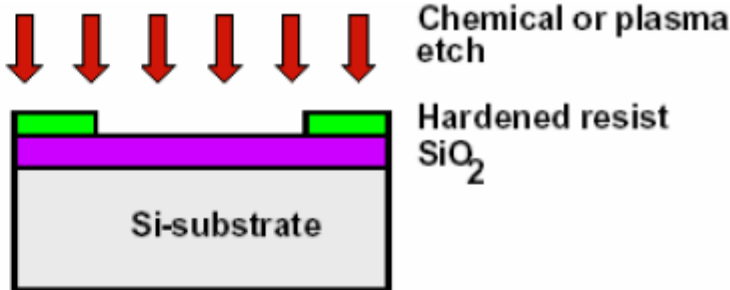
(d) After development and etching of resist, chemical or plasma etch of SiO 2
