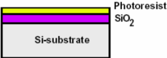
(b) After oxidation and deposition of negative photoresist
